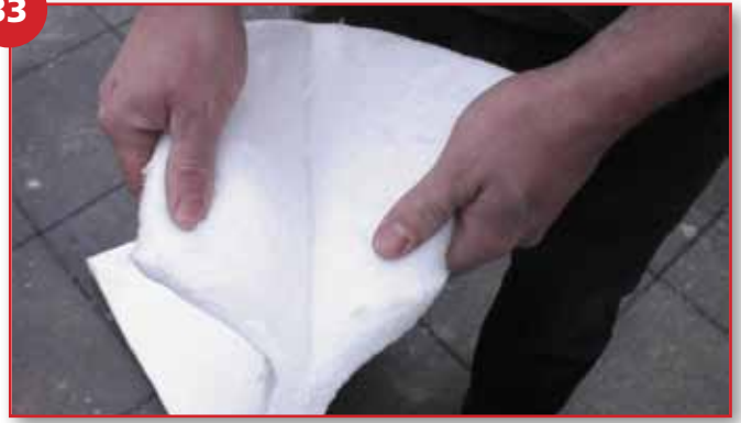
Split the thermal blanket supplied in half, do it slowly and make sure it peels apart evenly
